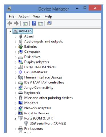
We recommend using the free serial terminal program "puTTY" to connect and test out commands, the serial port settings are: **115200bps**, **no parity**, **8 data bits**, **1 stop bits**. Command terminator is LINEFEED ("\n").
